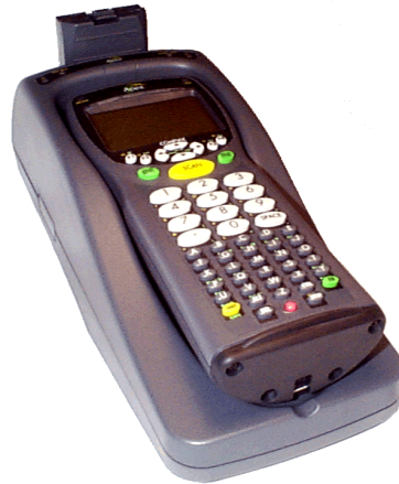
Figure 3-11: Apex III At Rest In Dock (Spare Battery Pack In Charging Slot)
