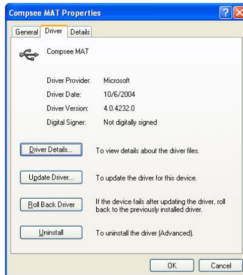
Figure 7 Driver details after installation is complete
